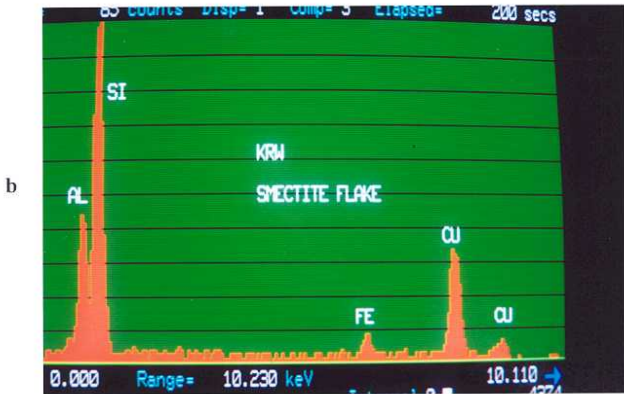
Figure 3a) Common authigenic calcite crystallites up to 5.0 microns in size; and a large smectite flake; and b) X-ray spectrum obtained from the smectite.
