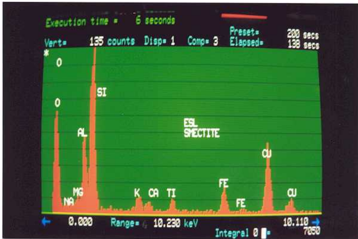
Figure 2a) A typical aggregate of smectite flakes in the sample; and b) its X-ray spectrum.
